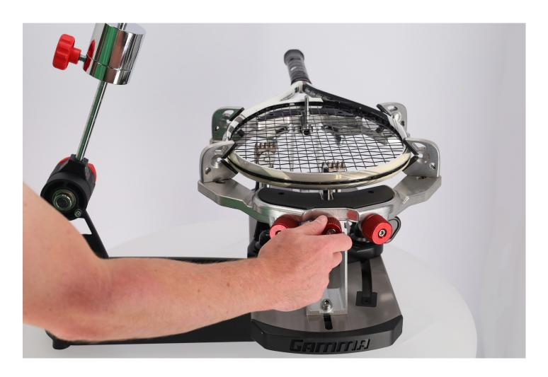
**CAUTION:** OVERTIGHTENING THE CENTER SUPPORTS WILL STRETCH THE HEAD OF THE RACQUET AND COULD CAUSE RACQUET DAMAGE.
