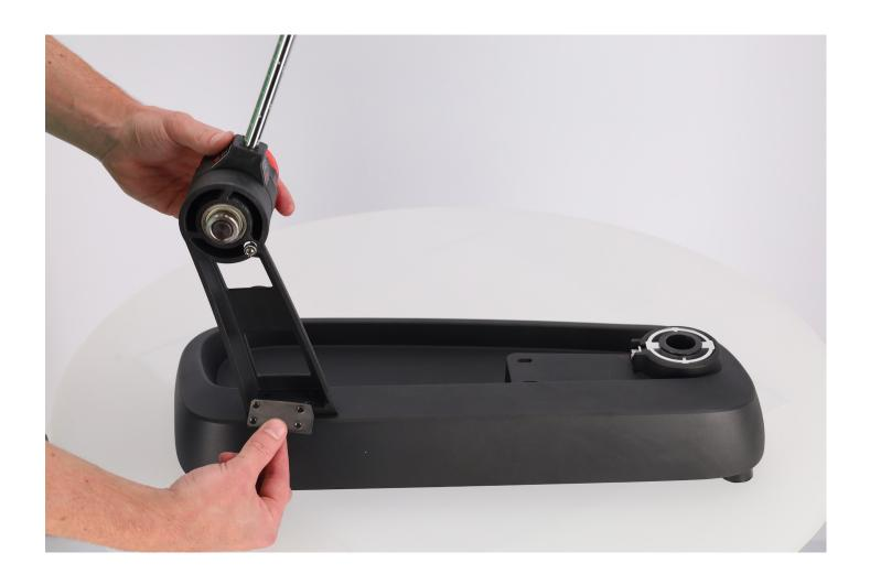
With the machine base on it's side, hold the winder stand in place while threading the 4 screws in from the bottom. Starting with the corners will make it easy to keep the winder stand and attachment plate aligned. After each screw is threaded, fully tighten each one to secure the winder stand.
