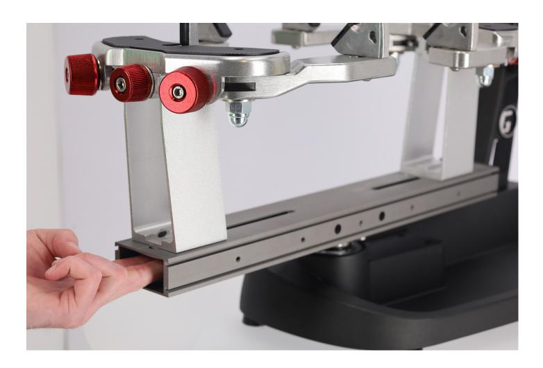
Install the mounting bolt through the support post and into the plate by hand and tighten with the 6 mm hex wrench.
