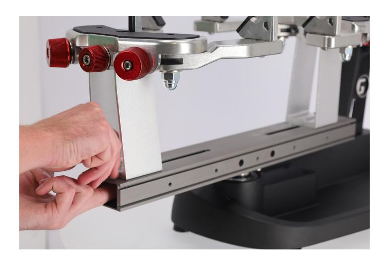
Re-install the turntable end caps. Repeat procedure on the opposite side of the turntable.
