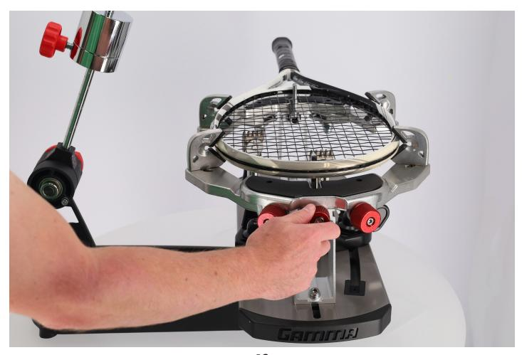
The frame shoulder supports are equipped with a bolt and spring for adjustment. This allows the user to picot the supports without having to readjust the bolt or lose security for the frame. Users can make adjustments as desired.
