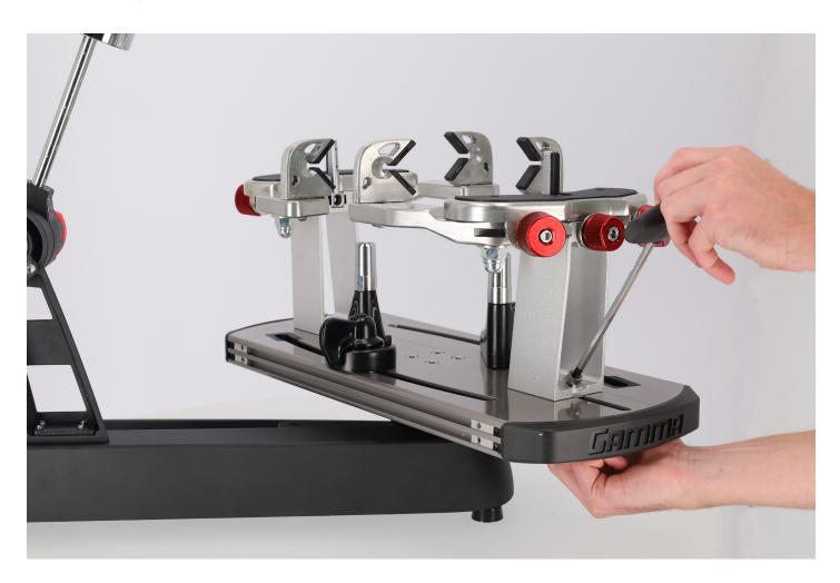
**CAUTION:** TO AVOID RACQUET DAMAGE, THE CENTER POSTS SHOULD NOT CONTACT THE RACQUET PRIOR TO LOCKING DOWN THE SUPPORT POSTS.
