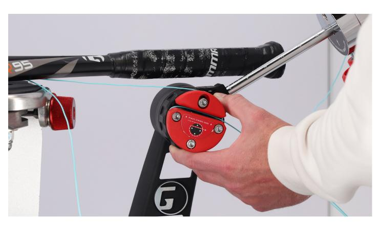
**WARNING:** TO AVOID INJURY, KEEP FINGERS AWAY FROM GRIPPER JAWS WHILE TENSIONING STRING.
